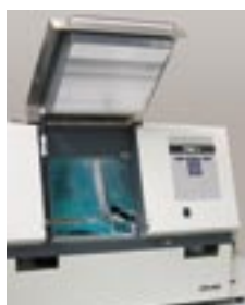
Device used to test UV exposure tolerance (UV-SUNTEST)
