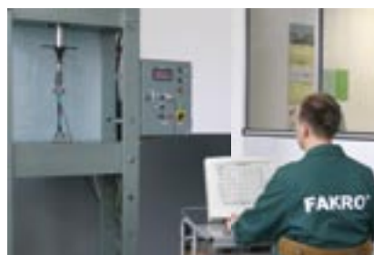
Testing the resistance of underlay to tear
